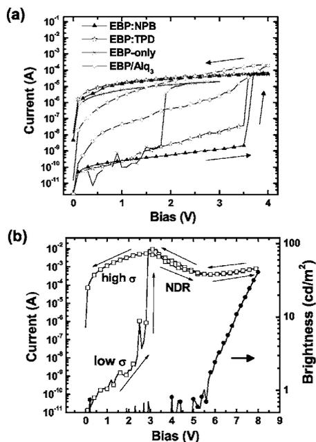
FIG. 2. (a)  $I$ - $V$  characteristics of polymer bistable devices. NPB and TPD with 0.08 wt % concentration are blended into the EBP films or an extra layer of  $\text{Alq}_3$  is inserted for carrier type study. (b)  $I$ - $V$ -luminescence characteristics of polymer bistable LED ( $\sigma$  represents the conductivity).
