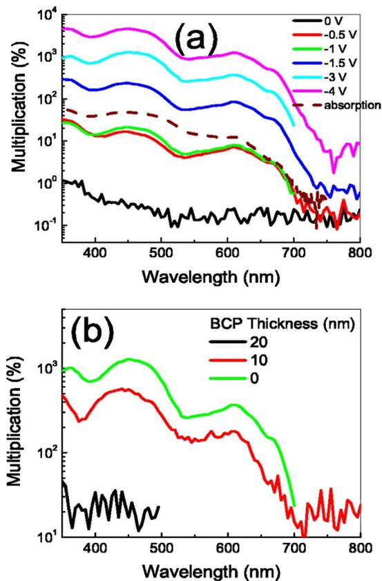
FIG. 4. (Color online) External quantum efficiency of devices (a) PEDOT (25 nm)/C<sub>60</sub> (80 nm)/BCP (8 nm)/Al and (b) PEDOT/BCP (0–20 nm)/C<sub>60</sub> (80 nm)/BCP (8 nm)/Al under various biases.
