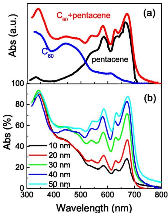
FIG. 2. (Color online) (a) Absorption of pure C<sub>60</sub> and pentacene and (b) absorption of solar cell devices with pentacene thickness in the range of 10–50 nm.
